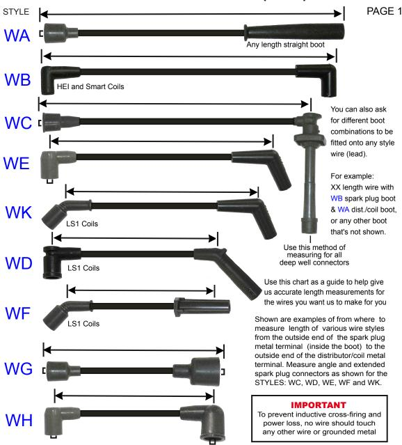
If the engine has no ignition wires installed to measure, to obtain accurate measurements, use some loose ignition cable or electrical cord to mock-up and measure a suitable route between spark plug top and the distributor/coil connection for each wire.
